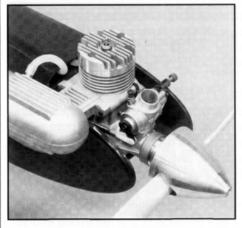
The engine shown here is an O.S. 61 SF, which is more than enough power for the Venture 60. Notice the vent line is hooked to the muffler for pressure. Notice also that the throttle cable is hooked to the throttle arm using a nylon clevis threaded onto a threaded coupler which is soldered to the steel throttle cable (phew!).
