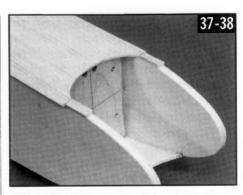
39. ☐ Sand the entire fuselage with a sanding block, starting with 80-grit sandpaper, then 150-grit. Round off the top and bottom corners as shown in the former cross-sections on the plans. Also, sand the rear edge of the top sheeting flush with the instrument panel and cut away the exposed portion of the tailpost at the stabilizer slot.
