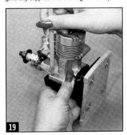
20. Temporarily bolt your engine to the mount, then mark the best spot on F-1 for the throttle pushrod to come through. The idea is to route the pushrod straight towards the carburetor's throttle arm. Remove the engine and mount, then drill at the mark with a 9/64" diameter drill bit.
