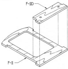
23. Using the fuselage top view on the plans as a guide, draw locating marks for the instrument panel and the headrest on the 1/8" lite-ply cockpit floor. Look ahead to photo 27 to see how the cockpit floor should be marked.
