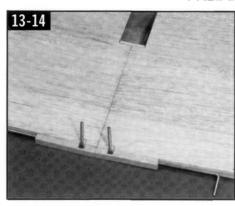
15. ☐ Score halfway through the center of the 1/16" x 1" x 3-3/4" plywood wing bolt plate, then gently crack it to match the dihedral angle. Glue the bolt plate to the bottom of the wing at the trailing edge. (See photo 33).
