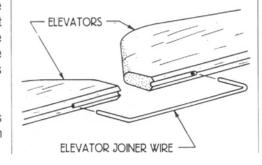
46. Temporarily tape the elevator to the back of the stabilizer, then use a sanding block to round off all of the edges. Sanding the stab and elevator at the same time insures that they will "flow" together perfectly at the tips.
