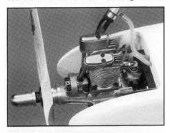
The engine shown here is a Saito .80, which is a good choice for the Flyin' King. Notice that the 14 x 6 wood prop is locked on by both the prop nut supplied with the engine and a high-quality, rounded Tru-Turn prop nut.
