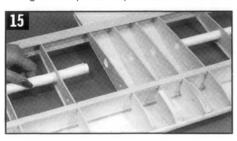
16. This is Important! Go back over every joint in the wing right now using medium CA glue, especially if you've been using thin CA to "tack" things together. When finished, you should be able to see a small build-up of glue on both sides of every joint. Remember that the strength of any wing is determined by the integrity of its glue joints.
