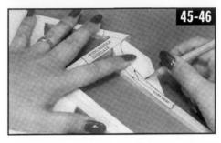
47. □ a. Due to the possible stretching of the plan during the reproduction process, the 1/8" lite-ply fuselage doubler may not line up perfectly all the way around with the balsa side. When gluing the doubler in place, it's most important to line up the rear edge of the F-2 notch with the back edge of SIDE-4. Use slow CA or epoxy to glue a doubler to each fuselage side. Avoid the classic mistake of making two left sides or two rights! You need one of each.
