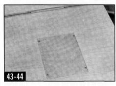
45. ☐ Now is a good time to give the wing a final sanding, starting with 150-grit, followed by 220- or 280-grit on a sanding block. Avoid the sheeting as much as possible. Concentrate on smoothing the major sheeting junctures, the tops of the fixed elevon pieces, the landing gear block, and the ends of the capstrips.
