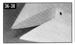
39. ☐ Again using a long sanding block, sand the entire length of the trailing edge so it's square with your building board as shown here.
