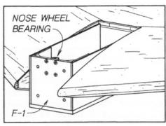
52. ☐ Glue the 1/4" x 1" x 3-1/2" balsa engine box cross brace, flush with the front surface of F-1. Use a sharpened piece of brass tubing to cut a clean hole in the cross brace for the nose wheel strut.
