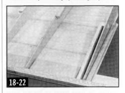
23. The slots for the two fins DO NOT run the full length of the sockets. Poke holes through the center sheeting (not the trailing edge sheeting) from the bottom in the fin slot area. Now you can use the holes as guides to carefully cut the slots. Use a thin sanding stick to finish off the slot edges. Extend the fin slots 1/4" back into the trailing edge sheeting. Trial fit the fins and continue trimming and sanding until satisfied with the fit.
