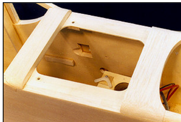
Above - Hatch removed. The hatch is held down at the back using two 10-32 nylon bolts threaded into plywood blocks under the lite-ply. A lite-ply tongue holds the hatch at the front. Below - 1/16" ply hardpoints are imbedded in top of hatch. The fuselage corners have all been sanded round.
