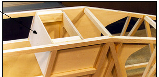
Fuselage Top showing the cabin rear and laminated wing blocks glued in place.
