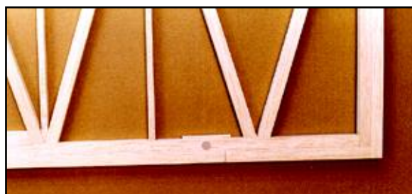
This Stabilizer Close-up shows the hard point and lite-ply reinforcement. Also notice the staggered joint at the corner of the stab
