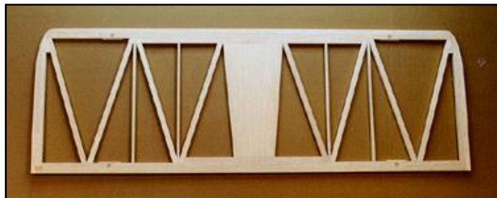
Complete Stabilizer ready for final sanding. The thin vertical sticks are 1/4" x 1/2" balsa added to help during the covering - that's where the green stripes overlap the other colors
