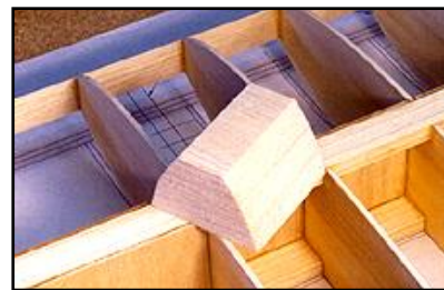
Above: A laminated balsa block trimmed to fit at the LE.
