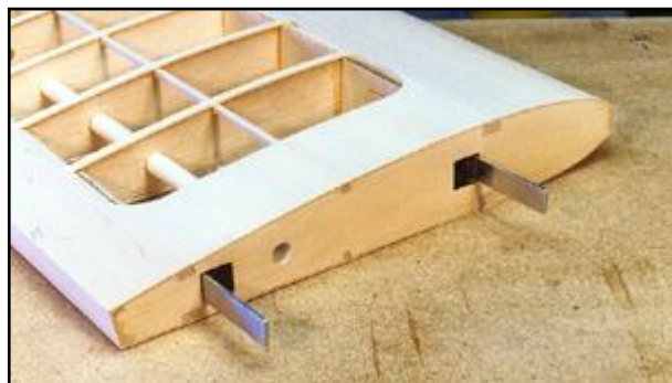
Finished Outer Wing Panel - The leading edge cap has been carved and sanded, and all of the sheeting has been carefully trimmed. Note the fillets in the corners of the wing joint sheeting. Not necessary, but it adds a touch of class
