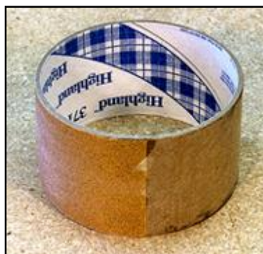
High-Tech Sanding Tool for sanding the fillets to a uniform curve. This is the cardboard core of a roll of shipping tape. Simply glue sandpaper to one half of it, and use the other half as a template for drawing the curves on your sheeting. Draw the curve, cut, and sand!
