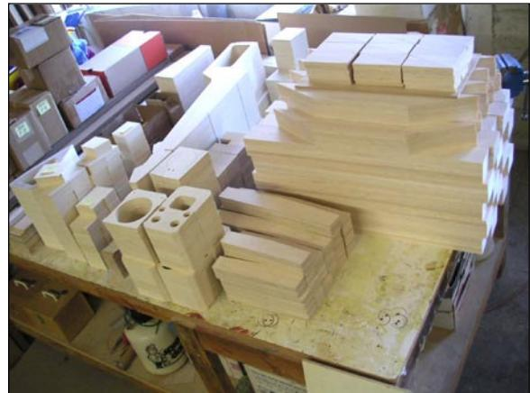
**Parts is Parts** – Here are just some of the finished parts for the R54 kit. The big stack on the right is balsa stabilizer parts. You can also see the two dihedral braces and a number of lite-ply parts including bulkheads, doublers, boat tail formers, wheel well frames, etc... Production quantity for the first run is 48 kits
